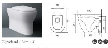
Cleveland BTW Rimless Pan with Ballina Seat. 36.9179.01 £430.00 Supplied with Chrome hinges, see more Type 1 hinges on **page 195.**
